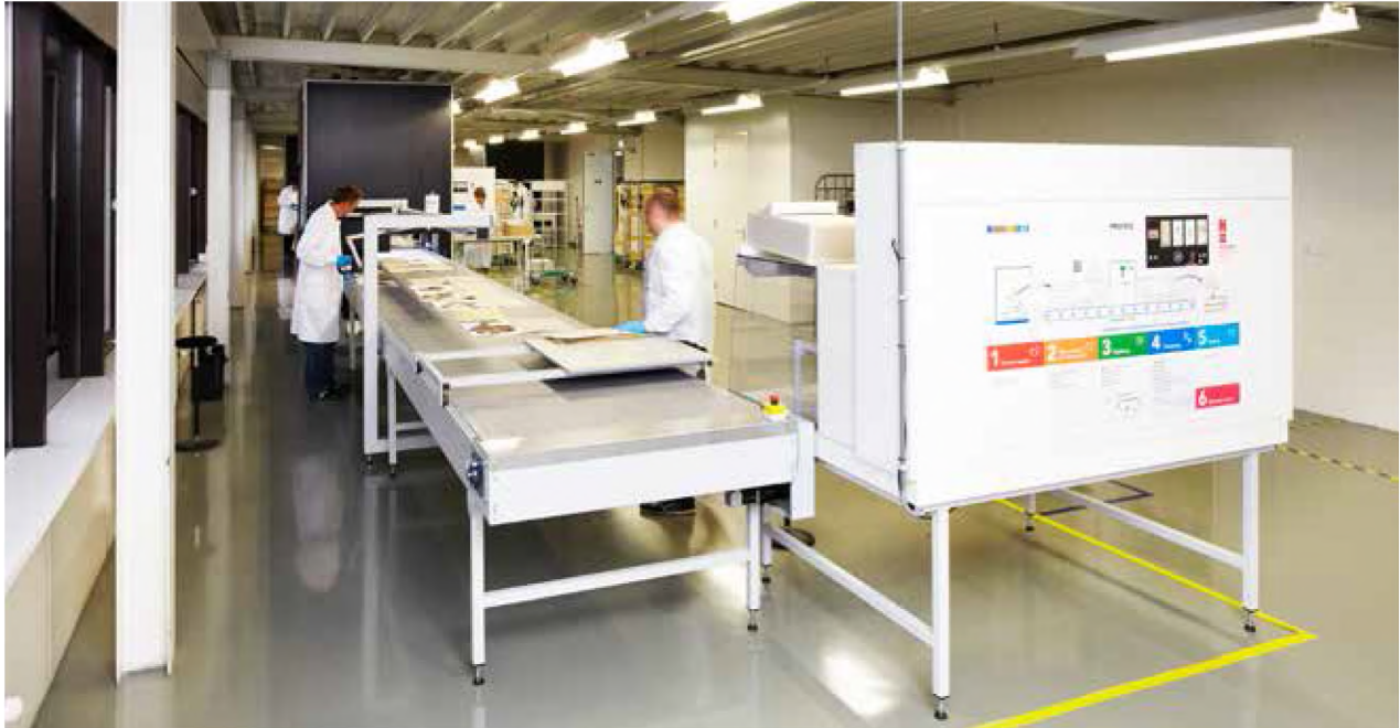
Fig. 6. One of the three assembly lines for photographing specimens. Shown is the beginning of the belt, where specimens and their folders are placed in two rows, halfway the QR codes are added (man with the black pistol-grip) and at the end, in the black box, the camera, which will only photograph the specimen row. The specimens are surrounded by buttons for colour calibration. Photo by the firm Picturae, reproduced with permission.
